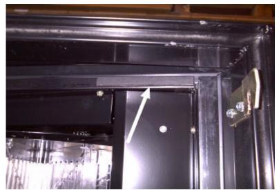
Attach Magnetic Gauge on the top of the mating strip as shown. This photograph displays magnetic strip attached for the right mating surface; the left side is attached in the same manner.
