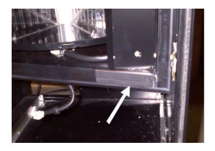
Install the larger magnetic gauges on the bottom gasket mating surfaces as shown
